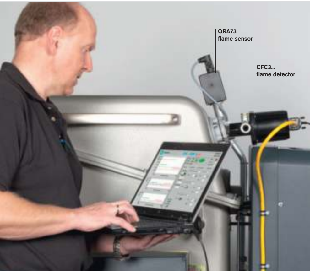
Testing and optimisation using a software tool
