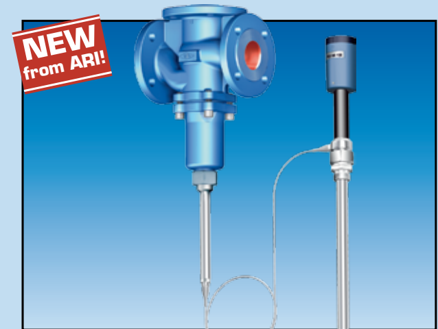
Thermal-opening valve (for cooling systems) opens with rising temperature
